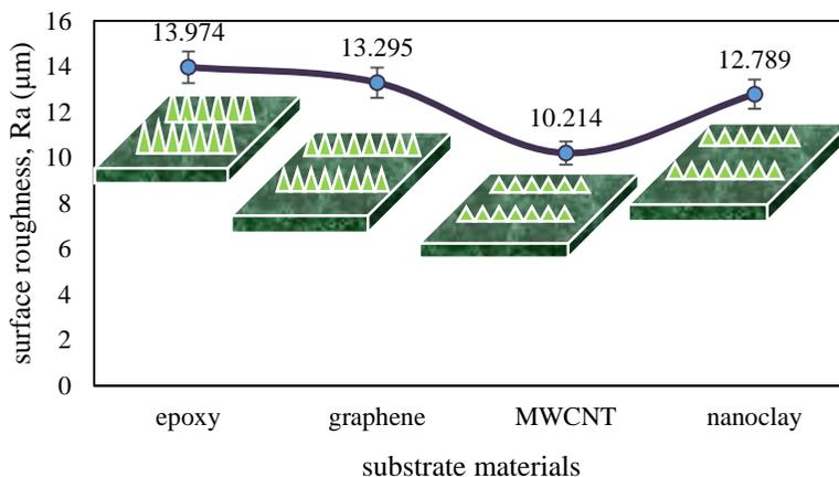
Figure 7: Surface roughness values of pistia substrates with schematic surface roughness images.
