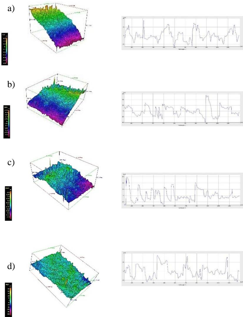
Figure 6: 3D isometric views of pistia substrates a) epoxy polymer, b) graphene-filled, c) MWCNT-filled and d) nanoclay-filled.
