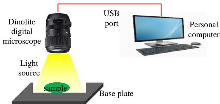
Figure 1: Schematic diagram of Dino-Lite Edge Digital microscope AM4815 series.
