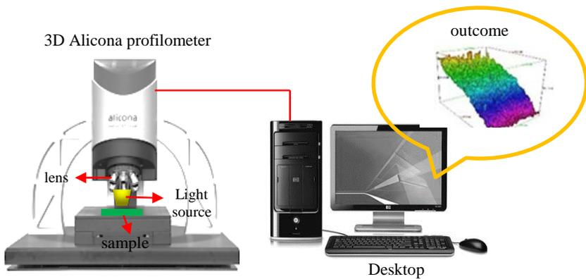
Figure 2: Schematic diagram of Infinite Focus Alicona profilometer surface topography machine.
