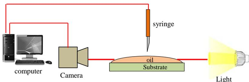
Figure 3: Schematic diagram of contact angle meter.
