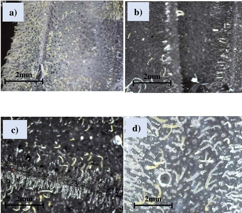
Figure 4: Digital microscope images of middle pistia substrates obtained by 3D Optical Noncontact Profilometer Alicona; a) epoxy, b) graphene, c) MWCNT and d) nanoclay.
