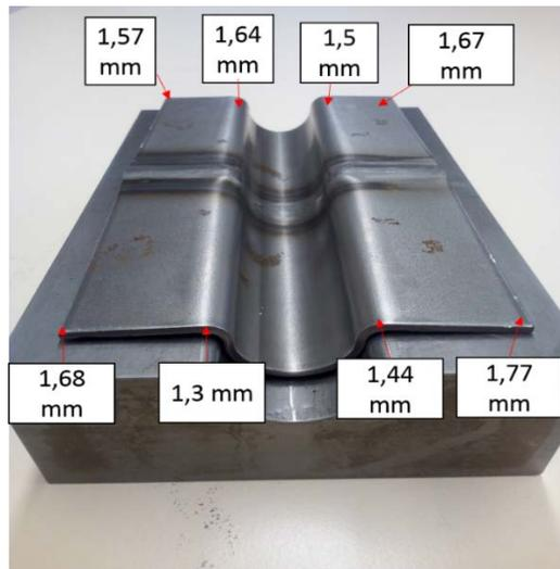
Figure 13: Experimental result of final deformation after coupled process welding-forming.
