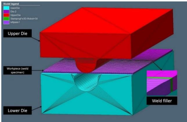
Figure 7: Details of forming components displayed in Simufact.Forming.
