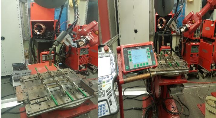
Figure 9: Robotic welding machine Comau Robotics SMART NS-16-1.65.
