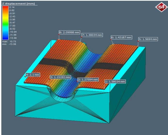
Figure 12: Virtual manufacturing simulation result of final deformation after coupled process welding-forming.
