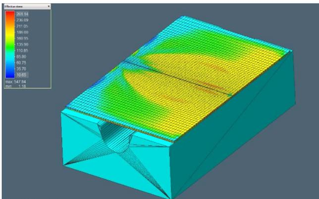
Figure 6: Transferred stress result from Simufact.Welding to Simufact.Forming.
