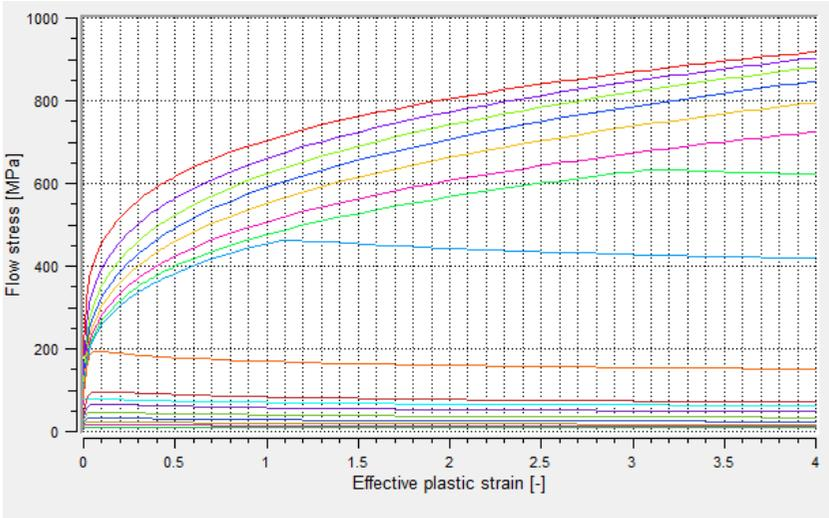
Figure 3: DC04 flow-curve.
