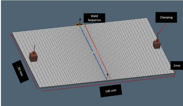
Figure 1: Details of butt-joint welding component displayed in Simufact.Welding.
