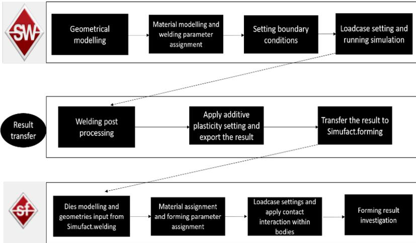
Figure 5: Process flowchart of coupled process welding-forming simulation using Simufact.Welding and Simufact.forming.
