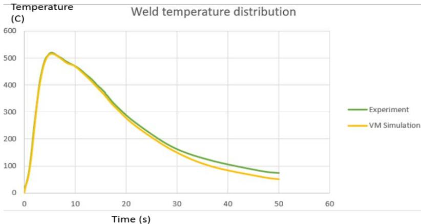
Figure 4: Comparison of temperature measurement between thermocouple result by experiment and temperature measurement of Simufact.welding.
