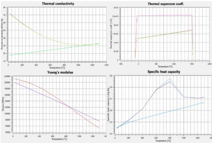
Figure 2: Temperature-dependant material properties of DC04.
