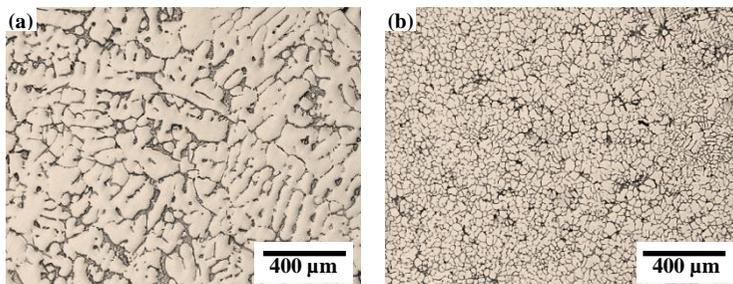
Figure 2: Optical microstructures (20X magnification) of Al4.8Si2.8Cu0.5Mg alloy (a) as-cast and (b) after the CS casting at a pouring temperature of 650 °C and cooling length of 400 mm
