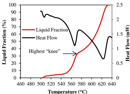
Figure 3: DSC heating flow and liquid fraction curves for Al4.8Si2.8Cu0.5Mg alloy
