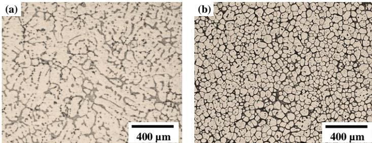
Figure 4: Optical microstructures (20X magnification) of Al4.8Si2.8Cu0.5Mg alloy subjected to partial remelting at 575 °C in an as-cast sample (a) and in a sample previously poured onto a CS with a cooling length of 400 mm and 650 °C of pouring temperature (b)
