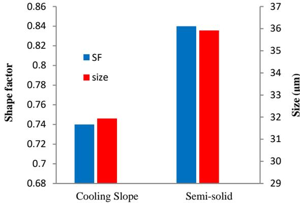
Figure 5: Variations in the SF and globule size of  $\alpha$ -Al particles after CS casting and subsequently partial remelting in a semi-solid state.
