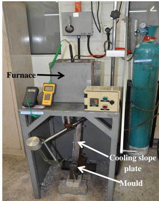
Figure 1: Cooling slope casting apparatus
