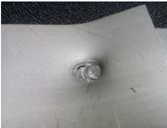
Figure 4: Pull out failure in sample with galvanneal metal
