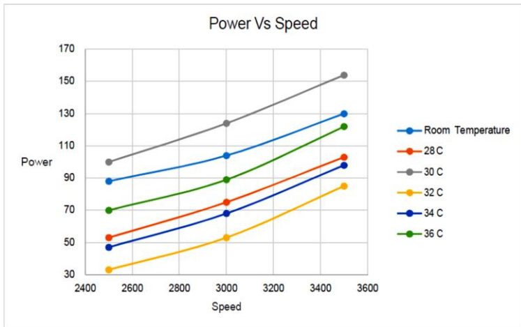
Figure 7: Power and speed for various fuel temperature
