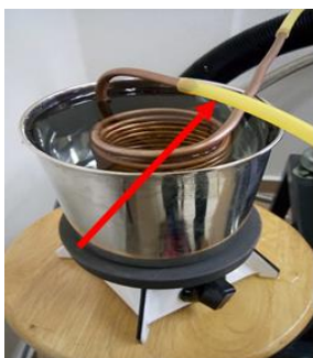
Figure 3: Fuel run through the heat exchanger heated using the electrical heater
