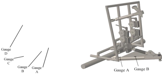
Figure 8. Strain gauge position (Left: Actual, Right: CAD Model)
