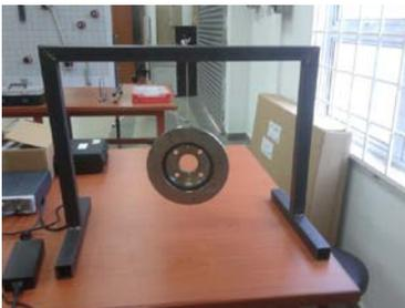
Figure 4: The brake rotor setup with free-free boundary condition
