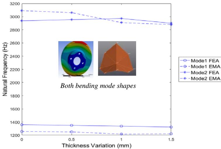
Figure 11: Comparison of FEA [5] and EMA for the natural frequency and thickness reduction
