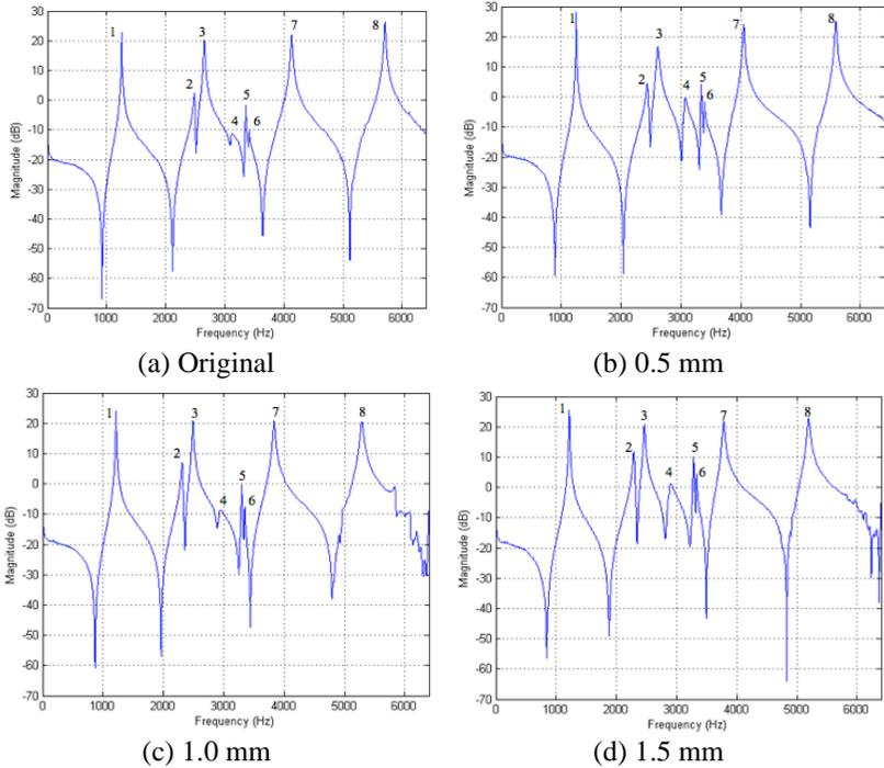
Figure 8: FRFs for thickness reduction
