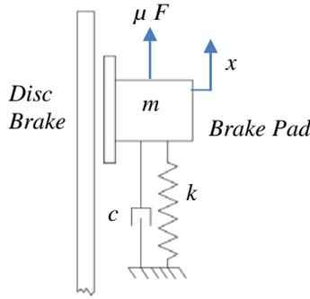
Figure 1: Schematic diagram of the disc brake and brake pad system
