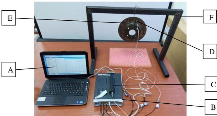
Figure 6: The experimental setup for impact hammer test. A) LMS Test.Lab; B) LMS Scadas Data Acquisition System; C) Brüel & Kjær Impact Hammer Type 8206-002; D) Brüel & Kjær Accelerometer Type 4514-001; E) Disc brake rotor; F) Hanging support.
