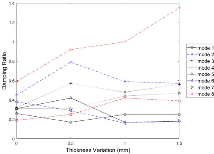
Figure 10: Damping ratio for different thickness reduction
