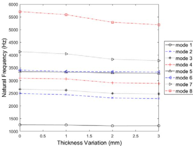
Figure 9: Natural frequency for different thickness reduction
