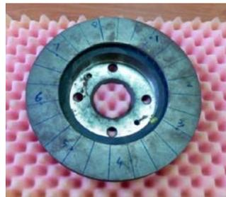
Figure 5: Point distribution of disc brake rotor.
