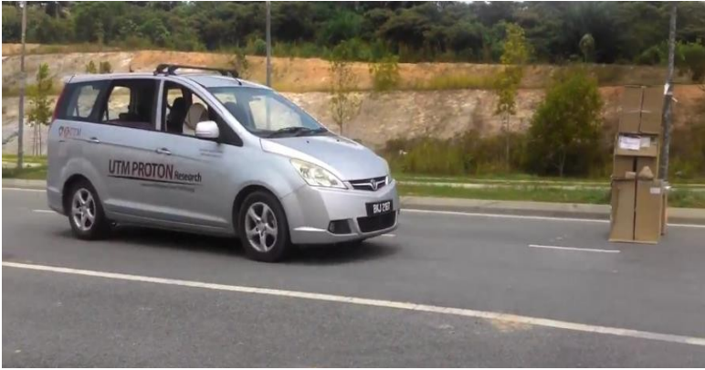
Figure 3: The configuration of the evasive lane change experiment.
