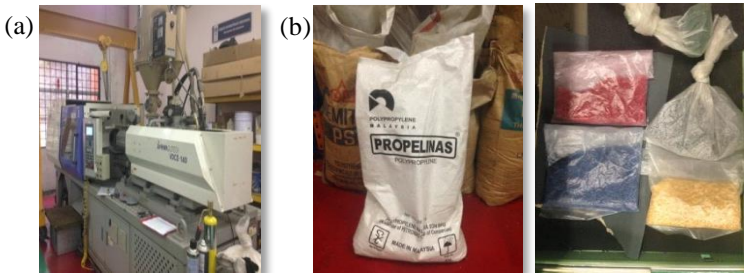
Figure 1: (a) Plastic Injection molding machine; (b) Polypropylenes (PP) white and colors used as raw material
