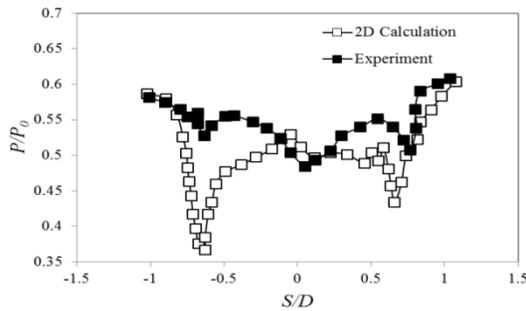
Figure 3 Trailing Edge Pressure Distribution comparisons
