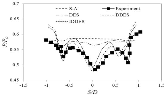
Figure 5 Trailing edge pressure distributions
