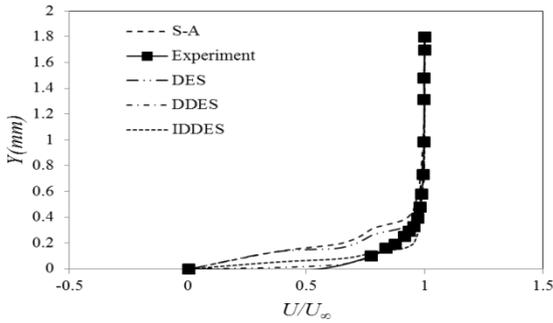
Figure 7 Boundary layer profiles at trailing edge (pressure side)
