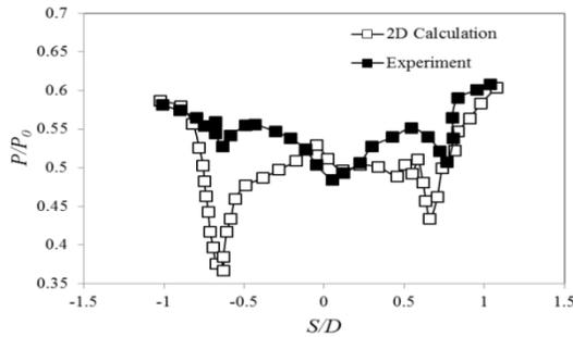
Figure 3 Trailing Edge Pressure Distribution comparisons
