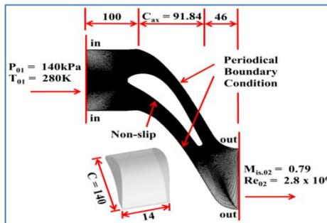
Figure 2: Simulation grid and boundary conditions
