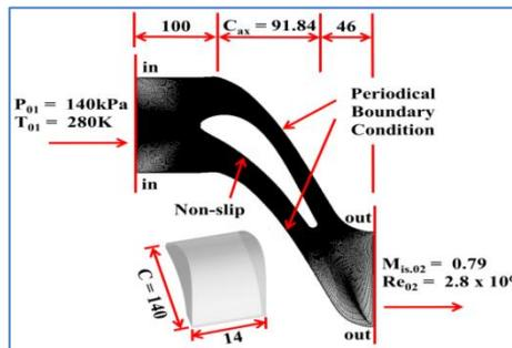
Figure 2: Simulation grid and boundary conditions
