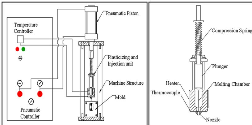
Figure 2: (a) Schematic of custom-made vertical injection moulding machine
