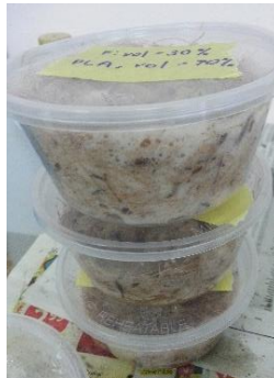
Fig. 3: The coir fibre was soaked in the PLA
