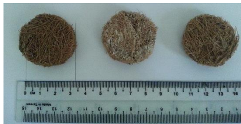
Fig 4: The specimens of coir fibre composite
