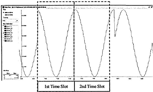
Fig. 14. Q for Channel 2 waveform start at 90° constellation point.
