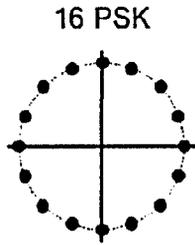
Fig. 2. Constellation diagram of 16 PSK.
