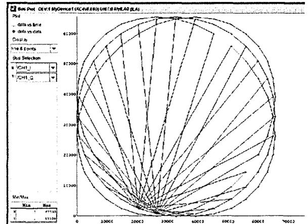
Fig. 19. Example of constellation diagram 16 PSK digitally plotted by Chipscope Pro Analyzer.
