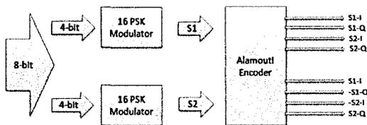
Fig. 6. 16 PSK Alamouti Block Level Architecture.
