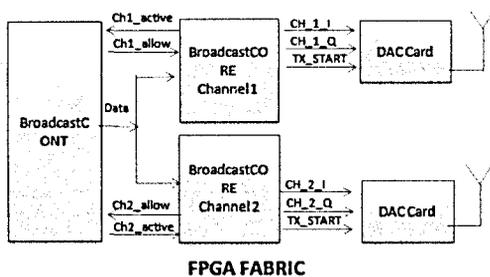
Fig. 7. 16 PSK Alamouti Encoder System Level Architecture.
