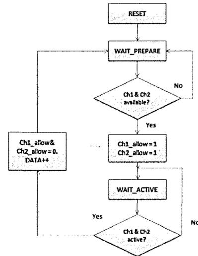
Fig. 8. Algorithmic State Machine for BroadcastCONT.
