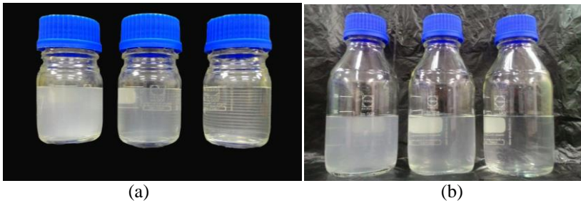
Figure 1: Photograph of the prepared nanoparticles of SiO 2 in HFE-7000 (a) First day of preparation, (b) 90 days of preparation (From left for both figures: 0.02%, 0.01% and 0.005% volume concentrations)
