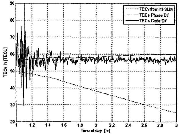
Fig.9(b) Comparison of TECs Code Different, TECs Phase Different and M-SLM TECv at KTPK station
