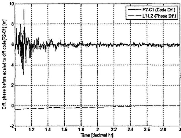
Fig.5(b) Different phase ( $L_1-L_2$ ) before scaled to different code ( $P_2-C_1$ ) at KTPK station.
