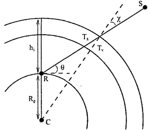
Fig.1. Geometry of Satellite-Receiver Link [3]
