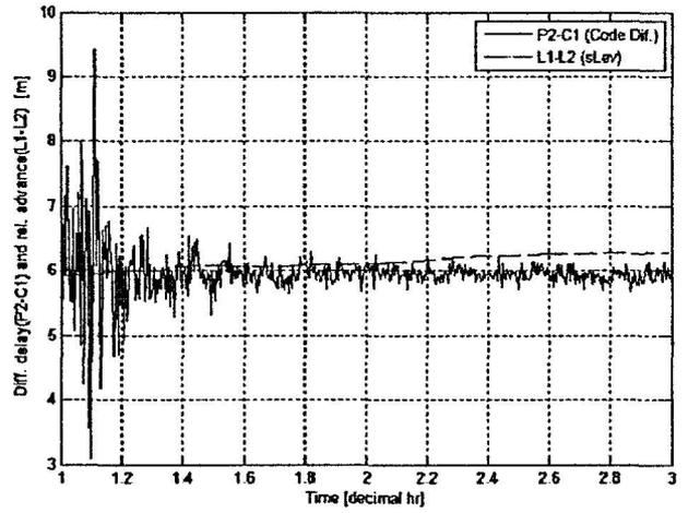
Fig.6(b) Relative range error computed from the differential carrier phase advance at KTPK station.
