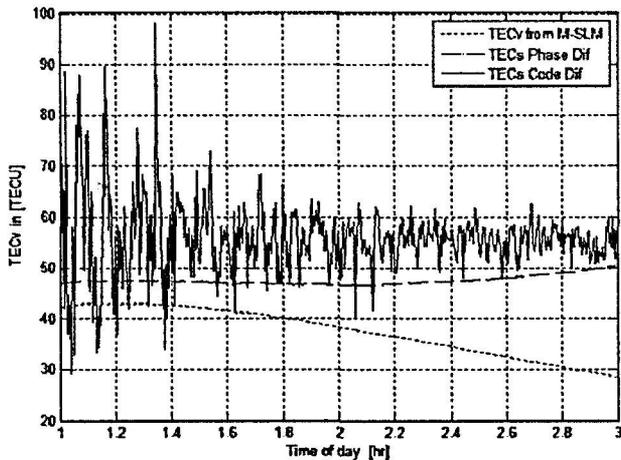
Fig.9(a) Comparison of TECs Code Different, TECs Phase Different and M-SLM TECv at UTMJ station
