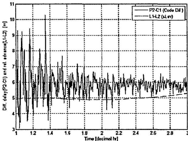
Fig.6(a) Relative range error computed from the differential carrier phase advance at UTMJ station.
