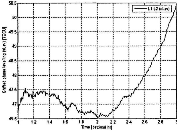
Fig.8(a) Shifted Phase Levelling (sLev) at UTMJ station
