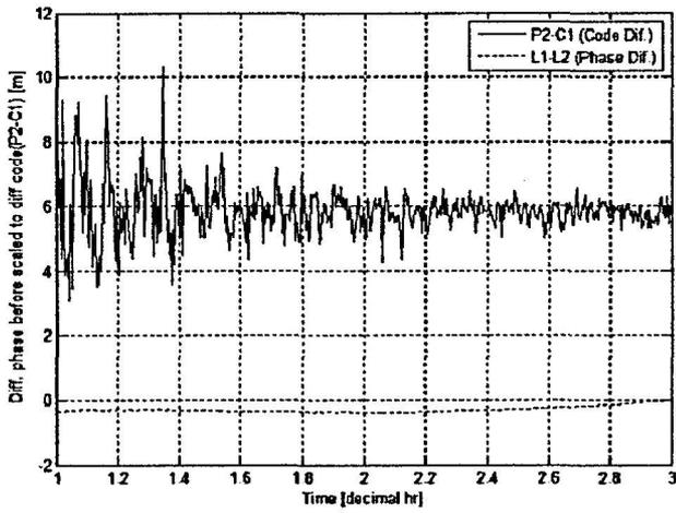
Fig.5(a) Different phase ( $L_1-L_2$ ) before scaled to different code ( $P_2-C_1$ ) at UTMJ station.
