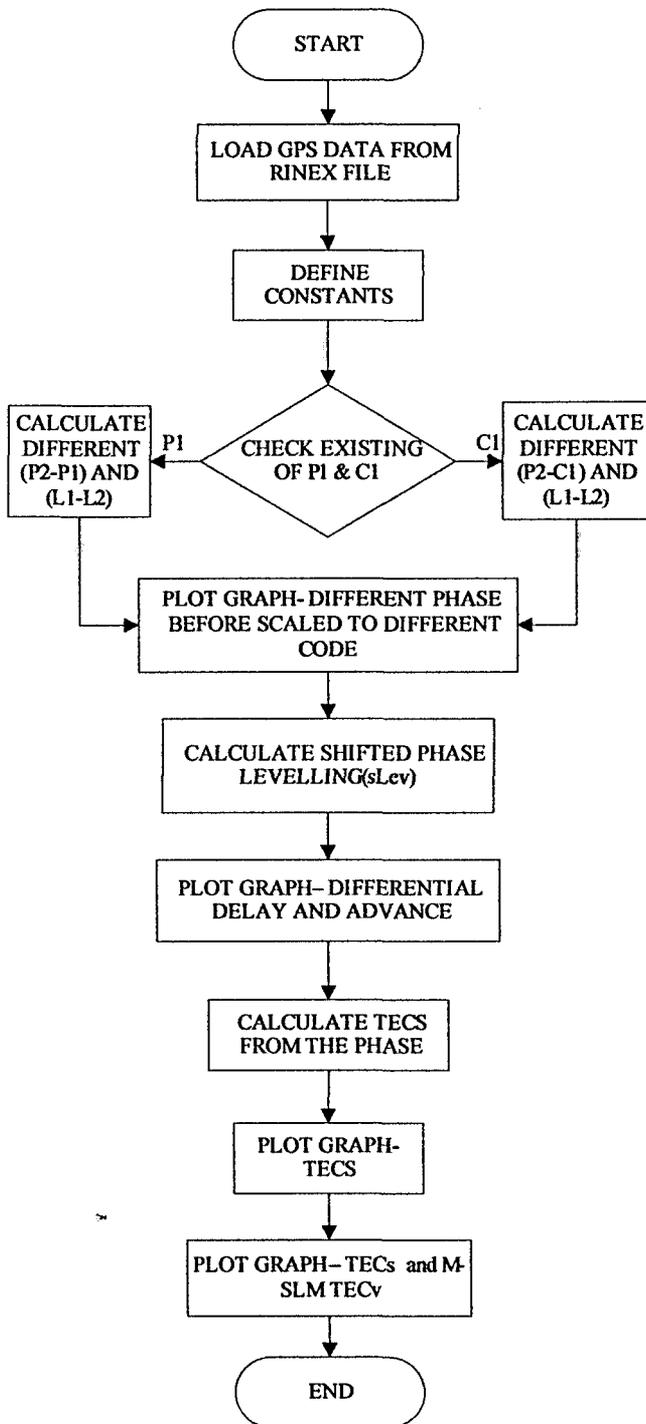
Fig.3. Flowchart process in Matlab simulation.
