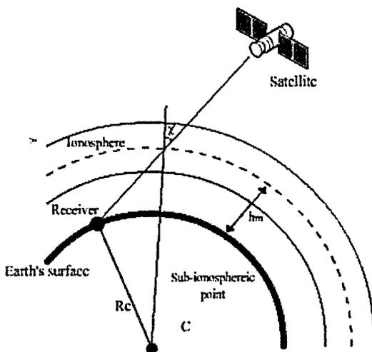
Fig.2. Ionospheric Single Layer Model
