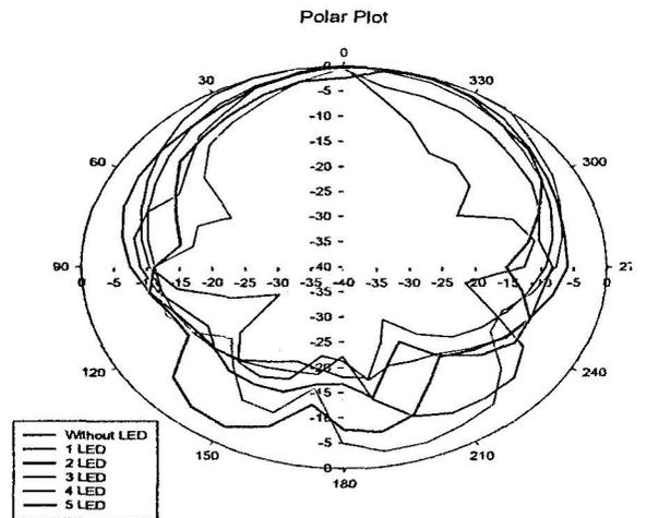
Figure 17: Radiation Pattern for all LED
