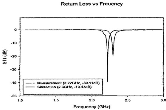
Figure 5: Return Loss vs Frequency Graph for Simulation and Measurement
