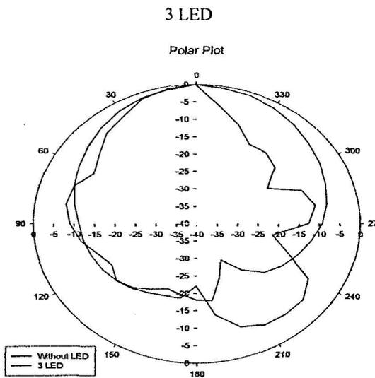
Figure 14: Radiation Pattern for 3 LED
