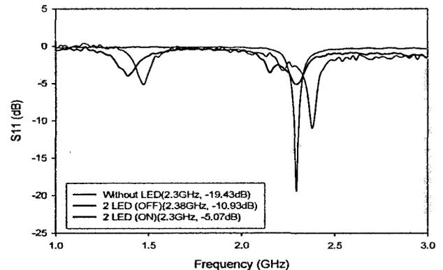
Figure 8: The Return Loss vs Frequency for 2 LED
