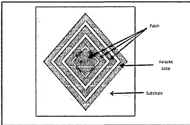
Figure 1: The Square Loop Antenna
