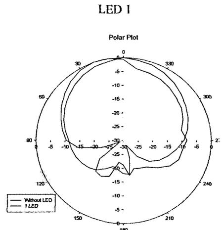
Figure 12: The Radiation Pattern for 1 LED
