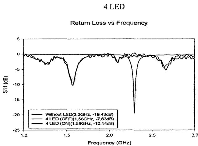
Figure 10: Return Loss vs Frequency for 4 LED
