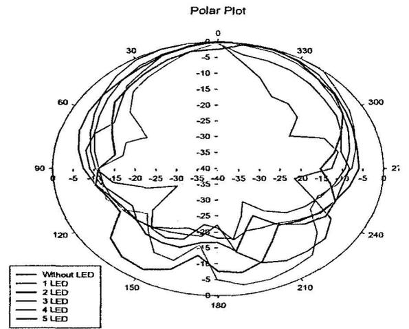
Figure 17: Radiation Pattern for all LED
