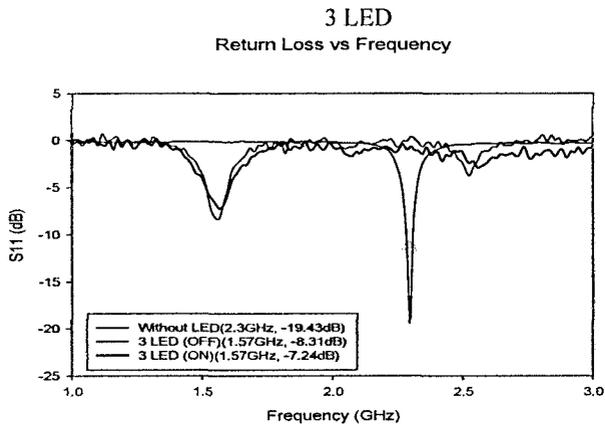
Figure 9: Return Loss vs Frequency for 3 LED
