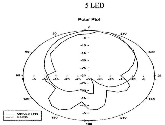
Figure 16: Radiation Pattern for 5 LED
