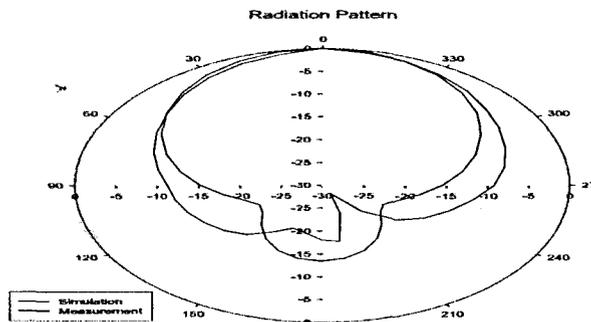
Figure 6: Radiation Pattern for Simulation and Measurement
