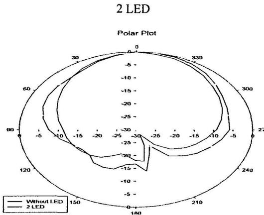
Figure 13: The Radiation Pattern for 2 LED
