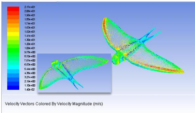
Figure 13: Velocity vector at  $\alpha = 0^\circ$
