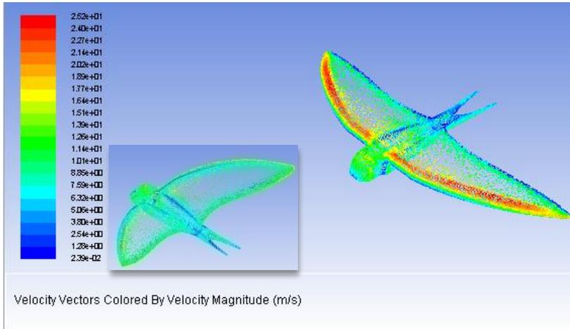
Figure 14: Velocity vector at  $\alpha=10^\circ$
