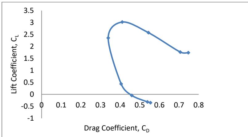
Figure 8: Simulation drag polar curve
