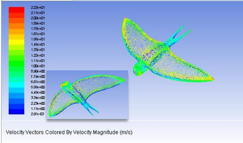
Figure 12: Velocity vector at  $\alpha = -10^\circ$
