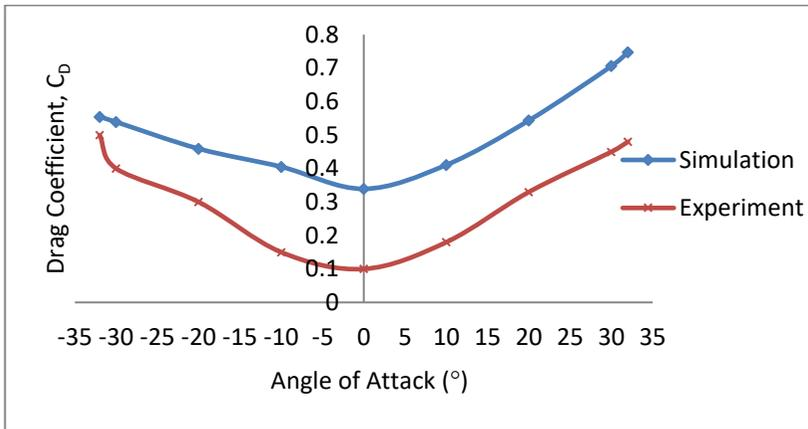
Figure 6: Drag coefficient curves
