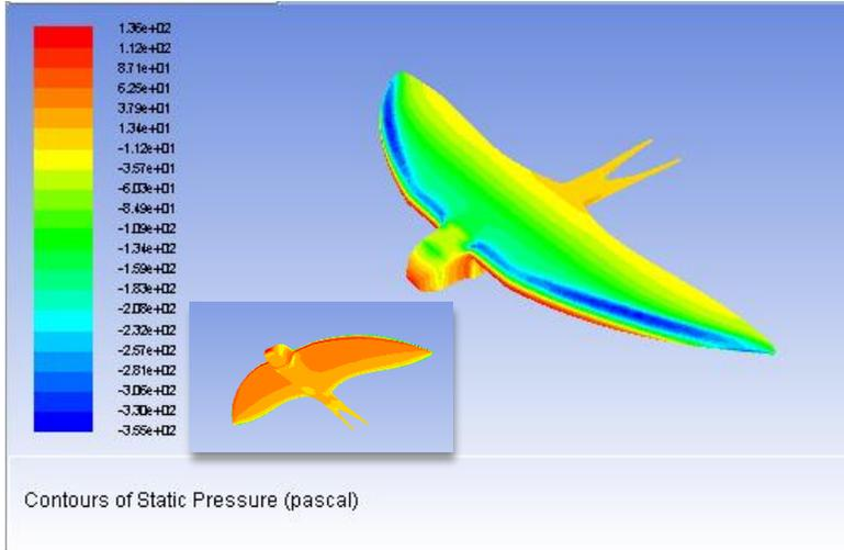
Figure 11: Pressure contour at  $\alpha= 10^\circ$
