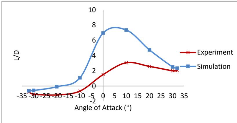
Figure 7: The lift to drag (L/D) ratio curves
