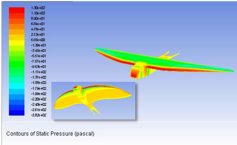
Figure 10: Pressure contour at  $\alpha = 0^\circ$
