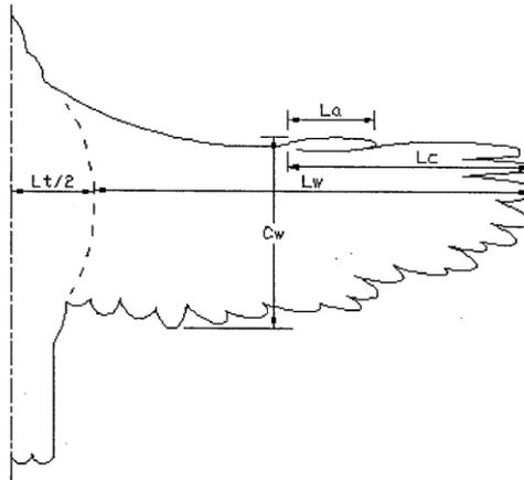
Figure 1: Bird's wing parameters [7]
