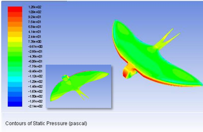
Figure 9: Pressure contour at  $\alpha = -10^\circ$
