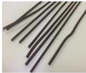
Fig. 4 Copper ABS Wire Filament by Single Screw Extruder Machine [12]
