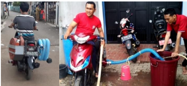
Figure 8: Firefighter motorcycle handling test
