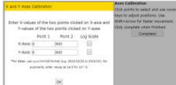
Fig.6. The process of setting the minimum and maximum value of x and y axis
