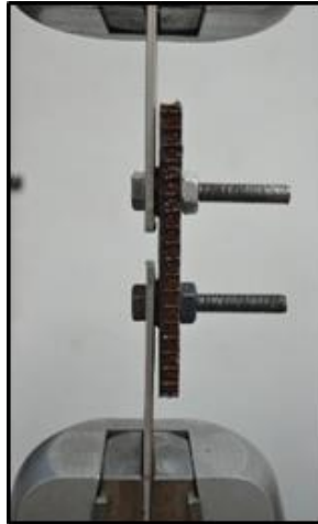
Figure 7: Shear test on hard point of CFRP honeycomb sandwich panel
