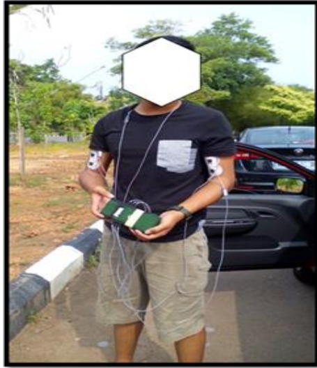
Figure 2: The EMG was set up at the subject's body
