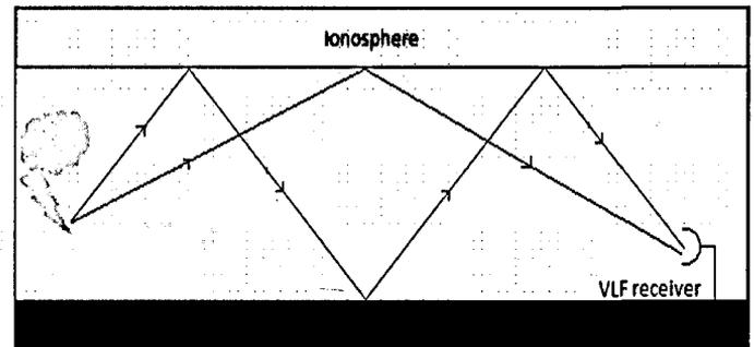
Figure 1: VLF wave propagation in EIWG.
