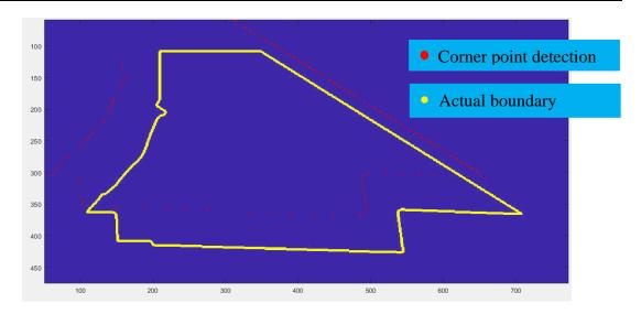
Figure 4 The corners point detected by Harris Corner Detection algorithms
