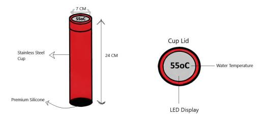
Figure 2.11: LED Flask
