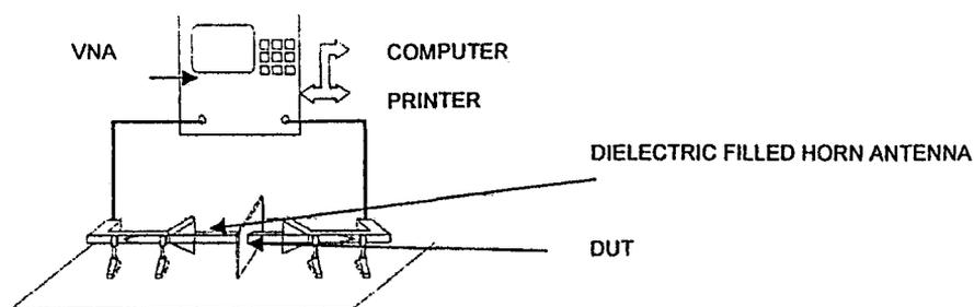
Fig 2. Rectangular Dielectric Waveguide Measurement (RDWG) System
