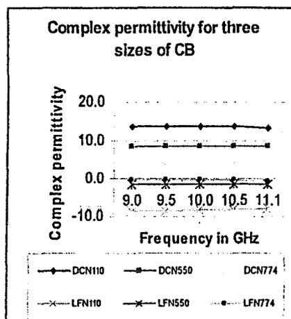
Fig 5. Graph of dielectric constant and loss factor for three particle size of CB
