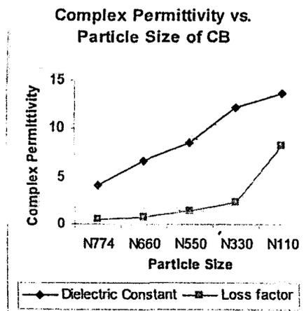
Fig 4. Complex permittivity for five different particle size of CB
