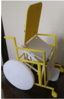
Figure 8: 3D printed prototype with standing configuration
