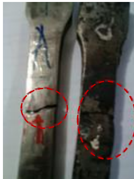
Figure 4: Cracking at sample 5th
