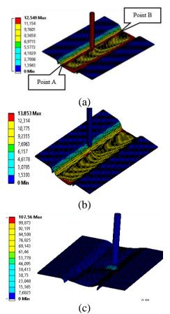
Figure 8 : SPIF simulation results of step down; (a) 2 mm; (b) 4 mm; (c) 6 mm
