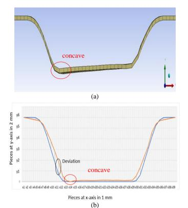
Figure 9 : Cross section profile : design = blue colour; product of SPIF = red colour
