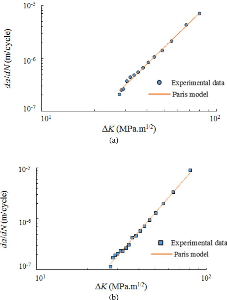
Figure 8: Fatigue crack growth curve described by the Paris model of (a) as-received and (b) dual-phase steels.
