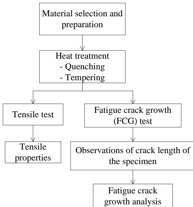
Figure 4: Process flow of the experimental procedure.
