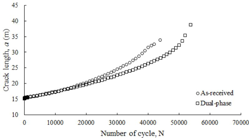
Figure 6: Fatigue life of as-received and dual-phase steels based on crack length observations.
