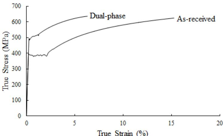
Figure 5: True stress-strain curves for as-received and dual-phase steels.
