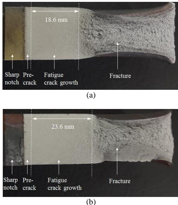
Figure 7: Fracture surface; (a) as-received specimen and (b) dual-phase specimen.
