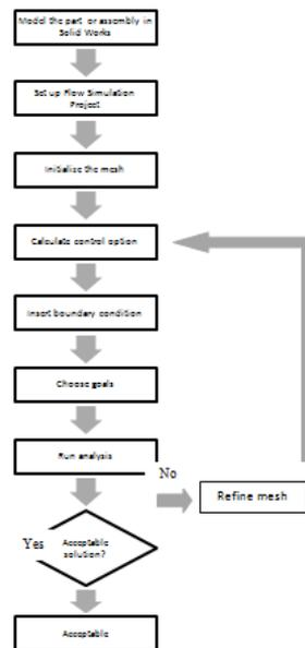
**Figure 2: The flowchart of flow simulation process**
