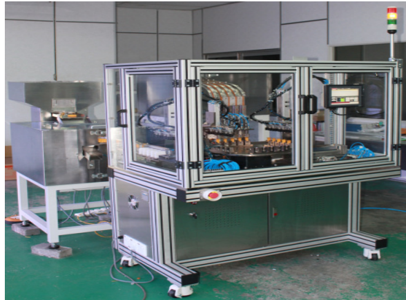
Figure 12 Constructed Automatic Roller Clamp Assembly Machine
