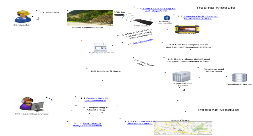
Figure 5: Proposed workflow for maintenance activity – PLUS
