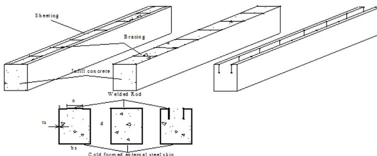
The inherent advantages of this system are derived from its structural configurations. Open box sections for beams will allow easy casting of in-fill concrete. TWC sections do not require temporary formwork for in-fill concrete as the steel acts as formwork in the construction stage and as reinforcement in the service stage.
