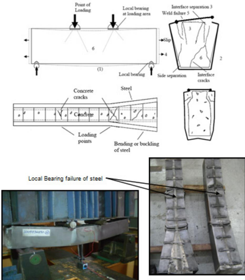
Figure 5: Failure Mode for CSWR50
