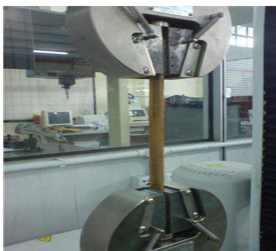
Figure 2A Specimen Was Loaded on a Instron 3366 Universal Testing Centre
