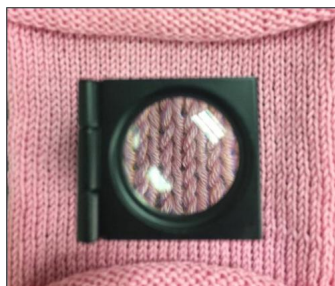
Figure 2: Stitch Counting on the Sample
