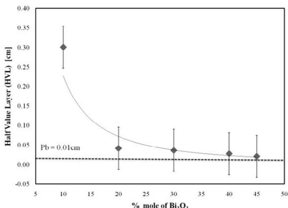
Figure 6: The Half Value Layer (HVL) of xBi<sub>2</sub>O<sub>3</sub> - (1-x)ZnO - 0.2B<sub>2</sub>O<sub>3</sub> - 0.3(SiO<sub>2</sub>)RHA glass samples compared to given value of Pb (0.01cm) using XCOM prediction program.
