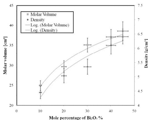
Figure 2: Molar Volume and Density of xBi<sub>2</sub>O<sub>3</sub> - (1-x)ZnO - 0.2B<sub>2</sub>O<sub>3</sub> - 0.3(SiO<sub>2</sub>)RHA glass samples.
