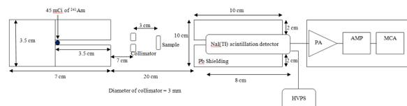
Figure 1: <sup>241</sup>Am gamma ray scattering experimental setup.
