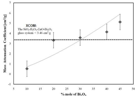
Figure 5: Mass attenuation coefficient of xBi<sub>2</sub>O<sub>3</sub> - (1-x)ZnO - 0.2B<sub>2</sub>O<sub>3</sub> - 0.3(SiO<sub>2</sub>)RHA glass samples compared to given value (3.46 cm<sup>2</sup>/g using XCOM prediction program.
