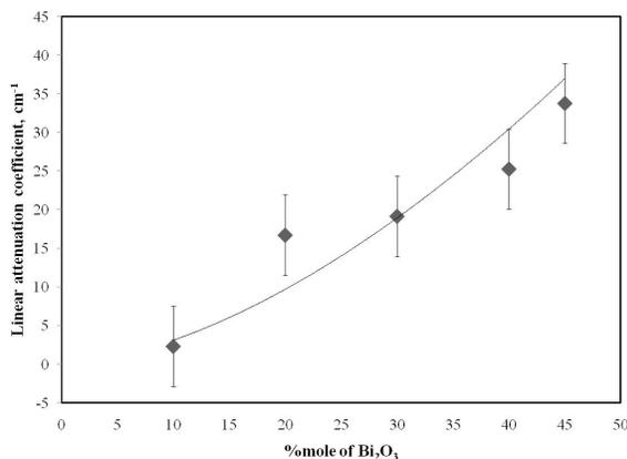
Figure 4: Linear attenuation coefficient of xBi<sub>2</sub>O<sub>3</sub> - (1-x)ZnO - 0.2B<sub>2</sub>O<sub>3</sub> - 0.3(SiO<sub>2</sub>)RHA glass samples.
