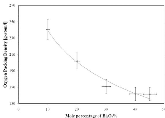
Figure 3: Oxygen Packing Density of xBi<sub>2</sub>O<sub>3</sub> - (1-x)ZnO - 0.2B<sub>2</sub>O<sub>3</sub> - 0.3(SiO<sub>2</sub>)RHA glass samples.
