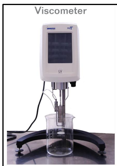
Figure 3.3 Brookfield digital viscometer used in viscosity test
