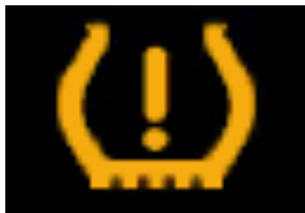
Figure 1.3: Tyre Pressure Monitoring System (TPMS) Indicator.
