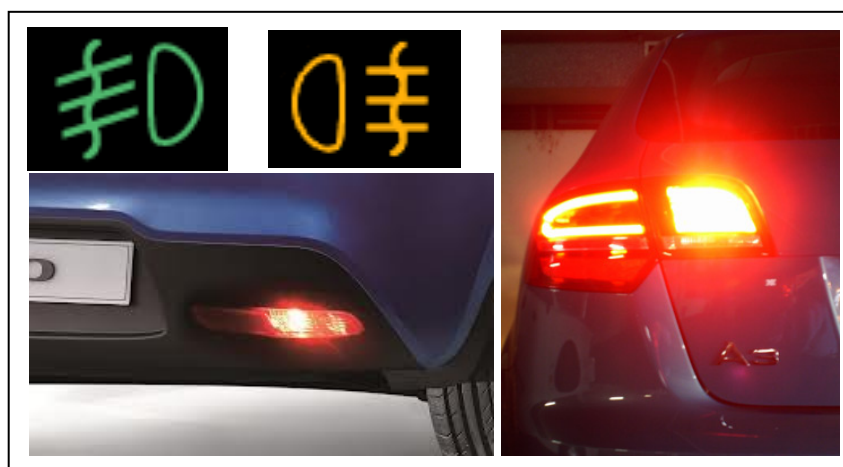
Figure 1.4: A symbol represent front fog lamp (left) and rear fog lamp (right) and, the position of the rear fog lamps on the car
