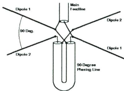
Figure 2: Wiring method of turnstile antenna
