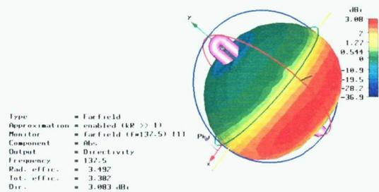
Figure 8: Far field at  $f = 137.5$  MHz for turnstile antenna
