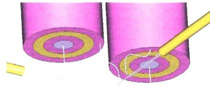
Figure 4: Connection of the dipoles to the phase line
