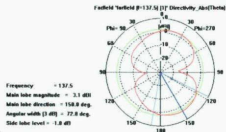
Figure 9: Radiation pattern for the turnstile antenna
