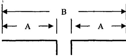
Figure 1: Basic half-wavelength dipole
