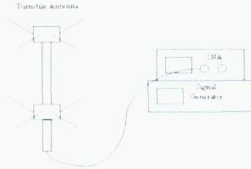
Figure 5: Connection for  $S_{11}$  measurement
