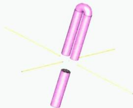
Figure 6: Turnstile antenna
