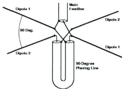
Figure 2: Wiring method of turnstile antenna
