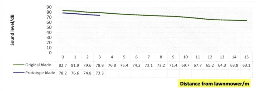
Figure 8: Comparison of both blades in the noise-distance test
