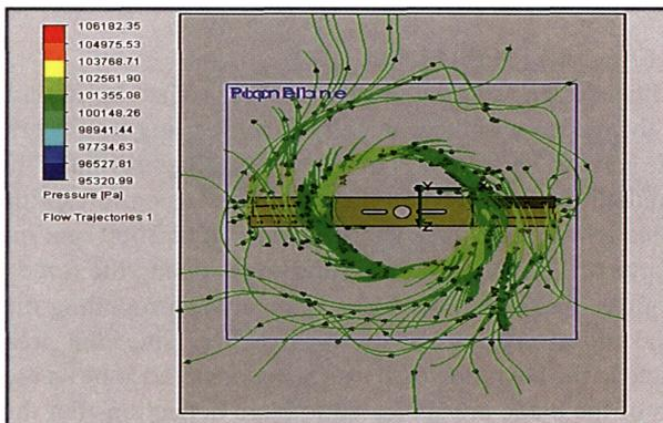
Figure 4: CFD trajectory of optimal design showing the pressures of the air particles
