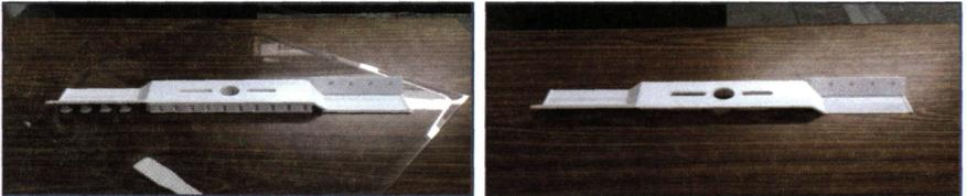
Figure 7: Fabricated prototype before and after support material removed
