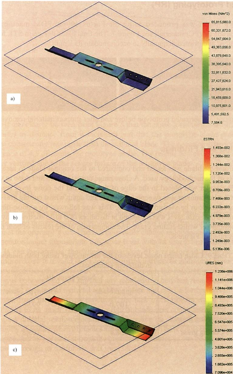
Figure 6: FEA results (a) stress distribution (b) strain distribution and (c) deflection
