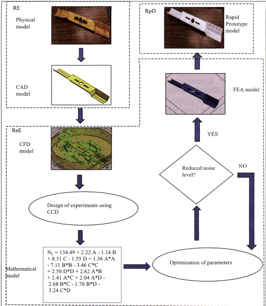
Figure 1: Integrated process flow for the design and development of a low noise intensity lawnmower blade
