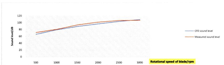
Figure 3: Comparison of the sound level from the virtual and physical results
