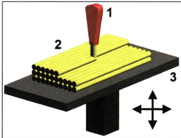
Figure 10: Deposition of material by FDM technology
