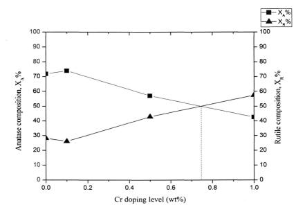
Figure 2: Proportion of anatase and rutile of pure TiO, and Cr-doped TiO,
