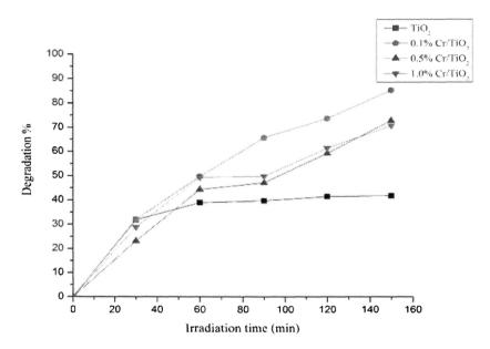
Figure 7: Degradation of methylene blue of pure TiO<sub>2</sub> and Cr-doped TiO<sub>2</sub>
