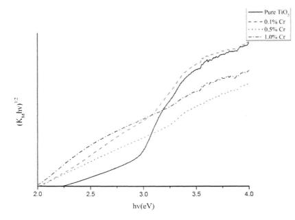
Figure 6: Tauc plot of pure TiO, and Cr-doped TiO,
