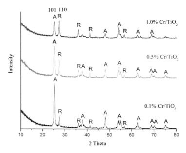
Figure 1: XRD patterns of pure TiO<sub>2</sub> and Cr-doped TiO<sub>2</sub>
