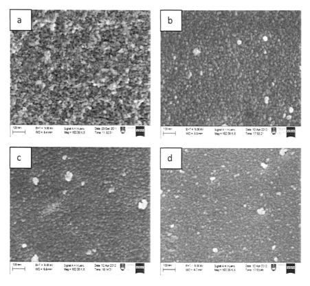
Figure 3: FESEM of pure TiO<sub>2</sub> and Cr-doped TiO<sub>2</sub>
