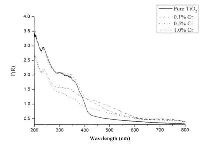
Figure 5: Kubelka-Munk absorption curves of pure  $TiO_2$  and Cr-doped  $TiO_2$
