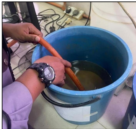
Figure 3.12 Removal of Excess Water Using the Siphoning Method.
