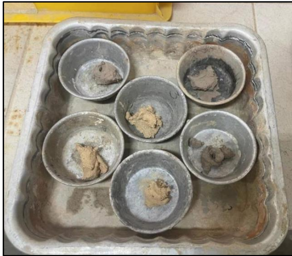
Figure 3.16 Liquid Limit Sample after Oven Drying
