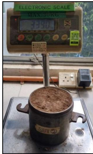
Figure 3.22 Weighing of Compacted Soil And Mould After Compacted
