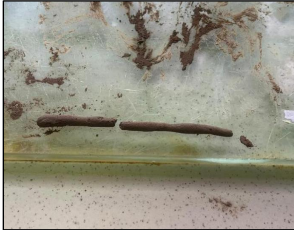
Figure 3.17 Crumbling of Soil Threads During Plastic Limit Determination
