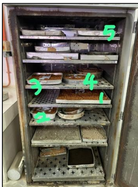
Figure 3.6 Oven Drying Process of Soil Sample
