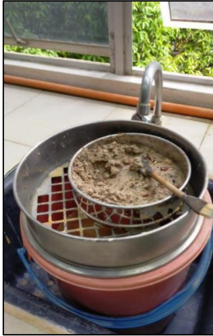
Figure 3.11 Wet Sieving Process for Separation the Fine Soil Particles
