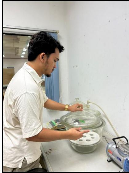
Figure 3.10 Desiccator Used to Remove Entrapped Air Bubbles
