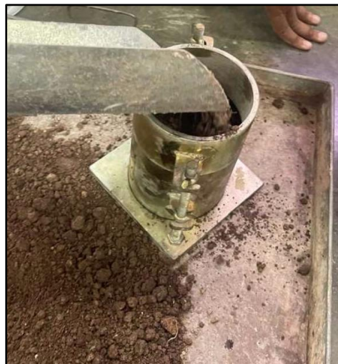
Figure 3.21 Standard Compaction Mould Used for Compaction Test
