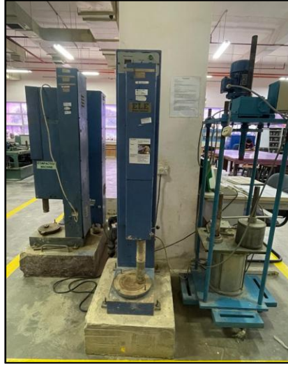
Figure 3.20 Automatic Proctor Compactor used for Standard Compaction Test
