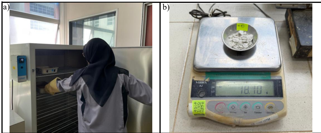
Figure 3.13 Post-Compaction Procedures (a) Oven-Dried Samples for 24 hours at 105°C (b) Recorded the Weight of Dried Samples
