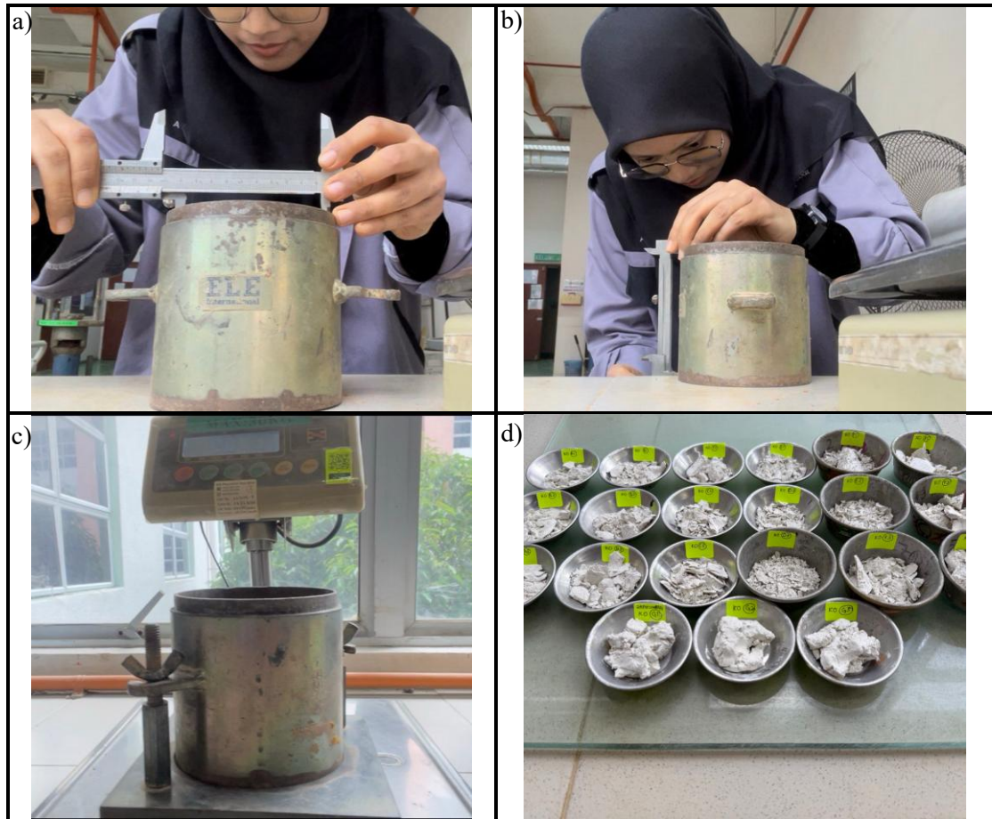
Figure 3.12 Procedures of Compaction Test (a) Measured Diameter of the Compaction Mould (b) Measured Height of the Compaction Mould (c) Weighted Compaction Mould With Base (d) Samples for Each Repeated Test of Compaction
