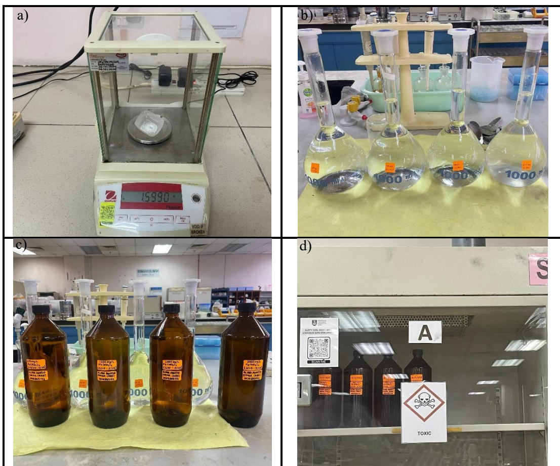
Figure 3.4 Preparation Pb(NO_3)_2 Solution (a) Weighted the Substance Based on Concentration (b) Dissolved the Substance Using 1000 mL Volumetric Flask (c) Stored the Solution in Glass Bottle With Proper Labelling (d) Keep the Glass Bottle in Specific Rack for Chemical Substances
