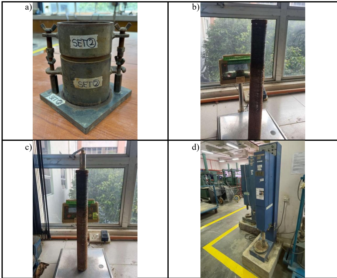
Figure 3.11 Apparatus for Compaction Test (a) Compaction Mould (b) Rammer for RPC and SPC (c) Rammer for MPC (d) Mechanical Compaction Machine
