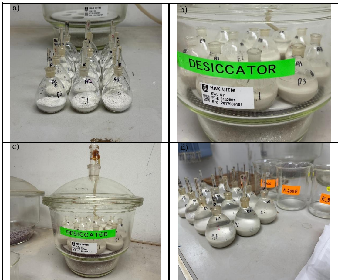
Figure 3.8 Specific Gravity Test (a) Sample Filled in 50 mL Pycnometer (b) Pycnometer Filled With Solution Until Almost Full (c) Pycnometer Left in Desiccator to Remove Air Bubbles (d) Pycnometer Filled With Solution Until Full and the Weight Were Recorded
