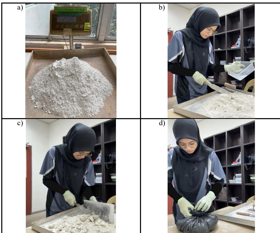
Figure 3.5 Preparation Sample (a) Weighted Kaolin Clay (b) Gradually Added Solution to the Soil (c) Mixed the Sample Until Well Mixed (d) Sealed Sample in Double Layers of Matte-Black Plastic Bag
