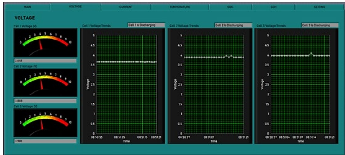
Fig. 6. The display of battery's voltage during both charging and discharging processes (in real time)
