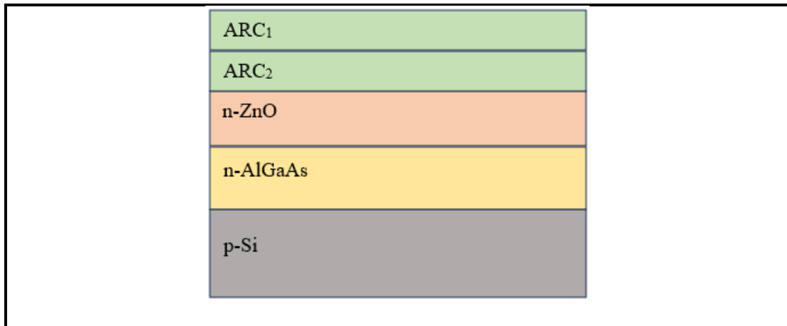
Figure 5.7 The Schematic Diagram of DLARC Configuration on ZnO/AlGaAs/Si Solar Cell
