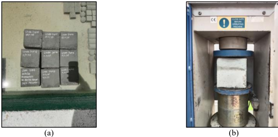
Figure 4: (a) Cube curing process and (b) Concrete compressive strength test machine
