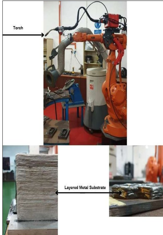
Fig. 4. Experimental setup for wire arc additive manufacturing.
