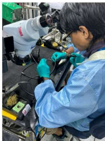
Figure 3: Repair of fiber Scope Using Soldering Technique
