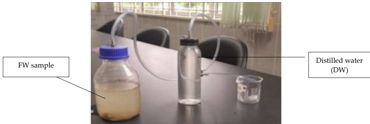
Figure 2. Determination of gas volume by water displacement technique
